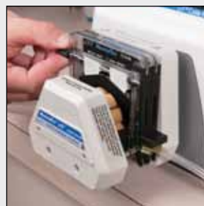
3. Adjust occlusion using index scale on cartridge.
