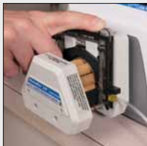
2. Snap cartridge into place on pump head.
