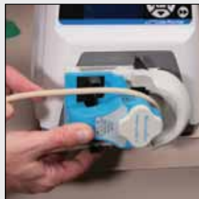
2. Place tubing over rollers and through retainers.
