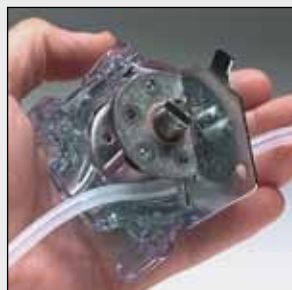
1. Disassemble pump head. Load tubing.
