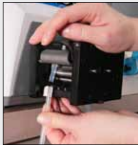
2. Hook left side tubing stop underneath retainer slot.
