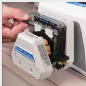
3. Adjust occlusion using index scale on cartridge.
