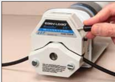
2. Close head. Adjust side tubing retainers to hold tubing.
