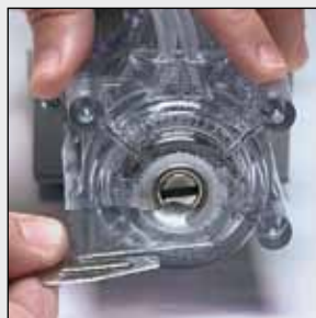
3. Reassemble two halves and mount on drive.
