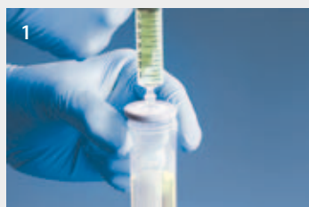
1. Stable fit on the filter on a 50 ml centrifuge tube
