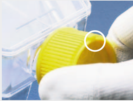
«VENT»-position at 12 o'clock = gas exchange
