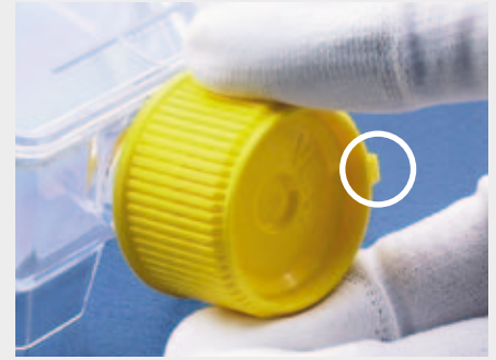
«VENT»-position at 3 o'clock = gas tight
