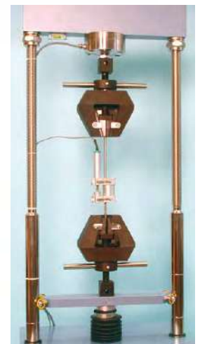
S205-05N + accessories for tensile test
