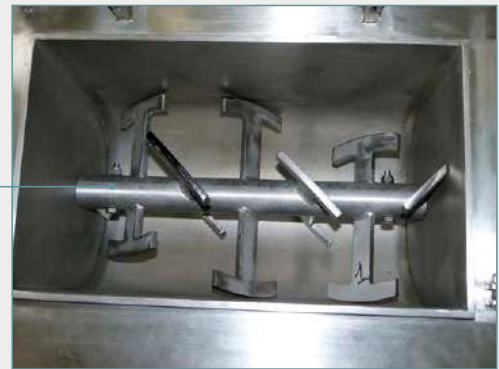
Detail: mixing shaft with helical blades
