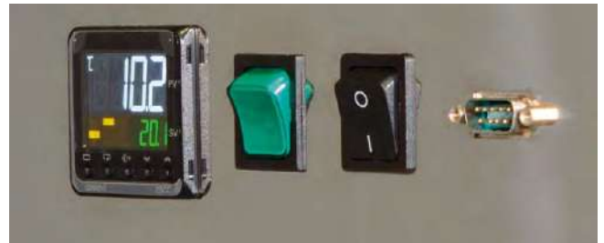
Cabinet switches and temperature controllers
