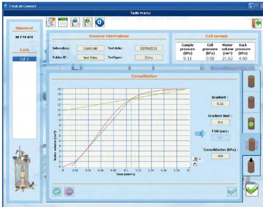
S335-10N Consolidation step in TriaxLab Connect
