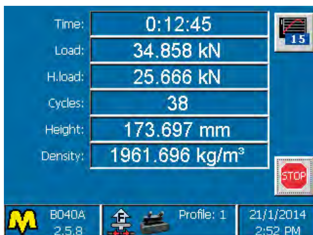
Test parameters during compaction
