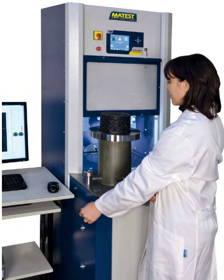
Test execution with shear stress measurement
