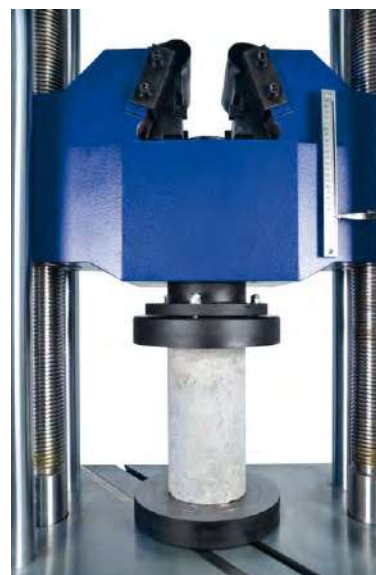
H001C-50 Detail of the standard compression platens
