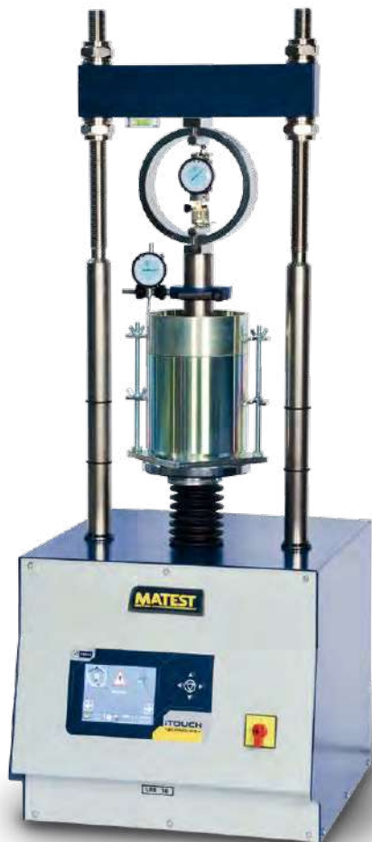
S212N with accessories for CBR test
