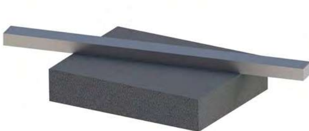
Optimally compacted sample with full planarity
