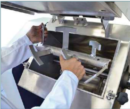
B026-05N Detail of the detachable mixing shaft
