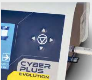
Unlimited memory storage with: 2 USB-Host ports* for PC, 1 SD card slot* (*memory hardware not included)
