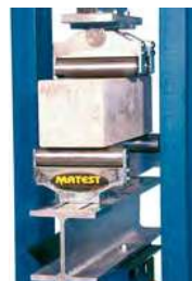
Flexure on concrete
