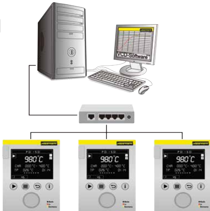
Example lay-out with 3 furnaces
