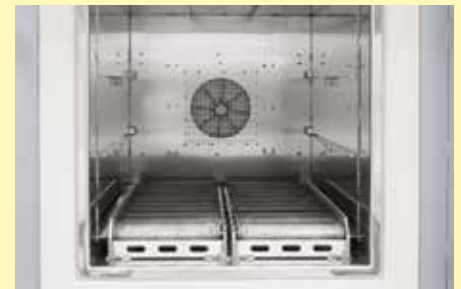
Roller conveyor in furnace chamber
