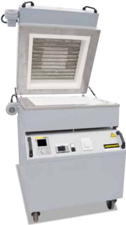
Fast-firing furnace LS 25/13
