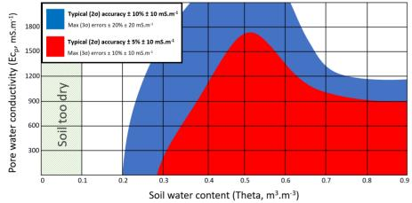
[1] The WET150 has been carefully optimised to provide accurate readings in soils and substrates - readings taken in water or air may not meet the full specification
