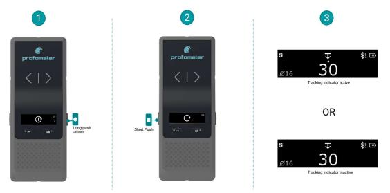
Figure 11: Activation or Deactivation of Tracking indicator
