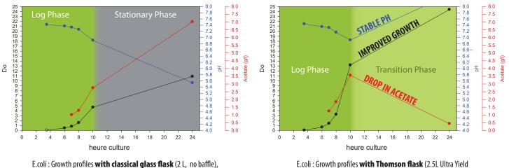
Flask, baffles), 500 mL Thomson medium, 400 rpm orbital shaker
