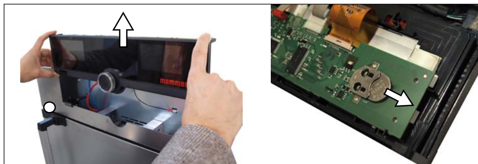
Fig. 32 Removing the lithium battery
