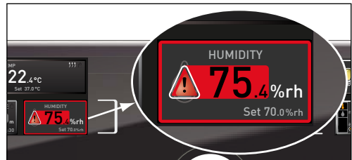
Fig. 21 Humidity monitoring triggered
