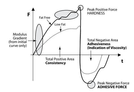
**DISCUSSION:** Once the trigger is attained, the force continues to increase until a surface fracture occurs. The modulus changes at this point to a less steep gradient, and the force nearly reaches a plateau.
