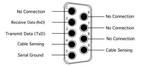
Pins 4 and 5 are used to sense presence of serial cable.
