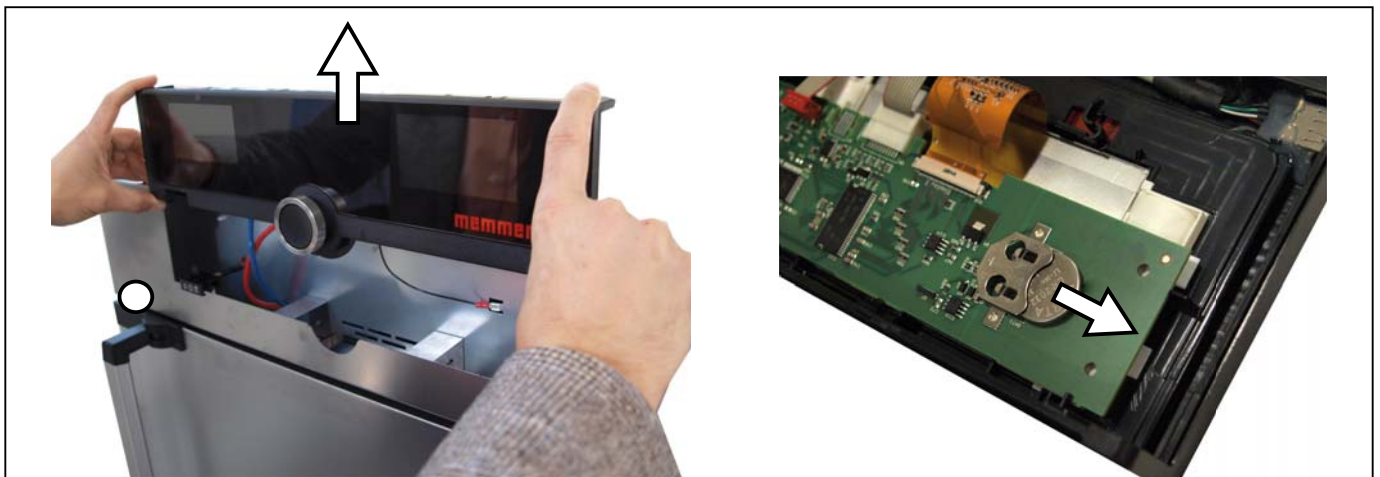
Fig. 23 Removing the lithium battery
