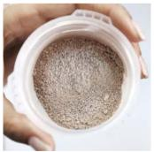
After grinding, a part of the sample will be analyzed. The remaining sample can either be discarded or it can be stored as a reference sample directly in the grinding chamber. In the later case, grinding chambers can be labeled and either stored in a refrigerator or in a drying room. Reference samples can be re-analyzed and traced at any time.
