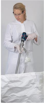
Quality assurance starts with the inspection of incoming goods! An all-layer sample of bulk goods is no longer a problem with PowderProof®, the sampler for powders and granules.
