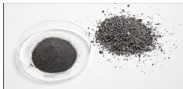
Ferrovanadium before and after grinding with the Planetary Mill PULVERISETTE 6 premium line
