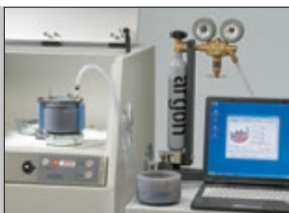
The PULVERISETTE 4 grinding in inert gas
