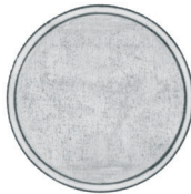
Erosion still permissible, plate can be polished
